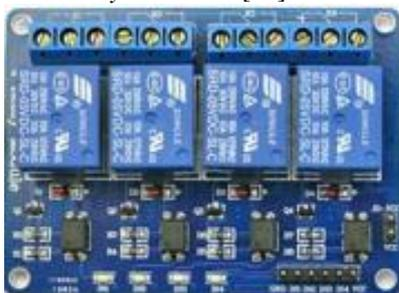
Gambar. 4 Relay 4 Channel
